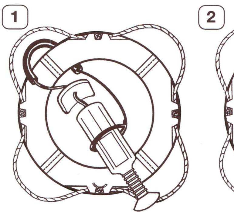
**1.** Put the line around the lifebuoy and thread the holder <u>and</u> foam padding through the loop.
